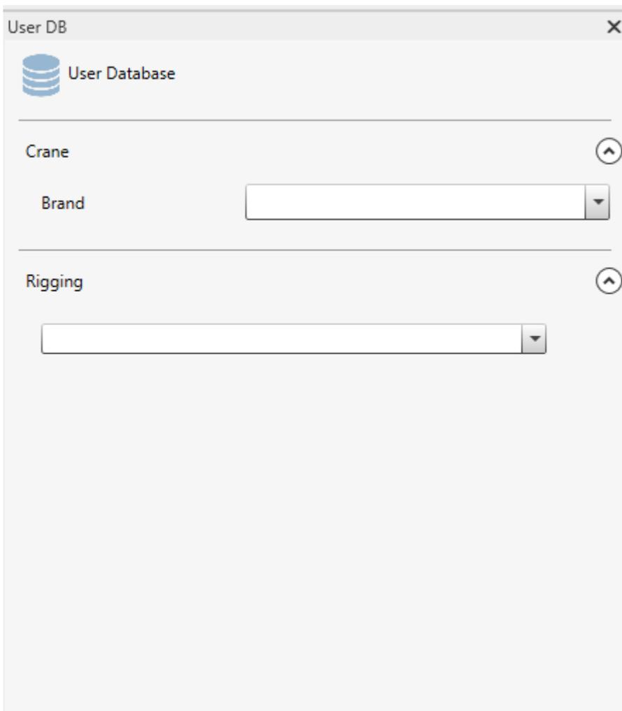
Under crane you can create/edit/delete load charts and crane engines properties.
